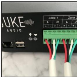
Plug each connector firmly into the Juke until it locks in place
