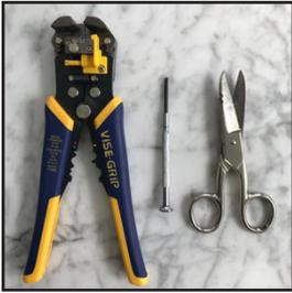
Tools required (not included): wire strippers, scissors and small blade screwdriver
