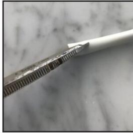
Cut a small amount of the insulation covering the speaker wires
