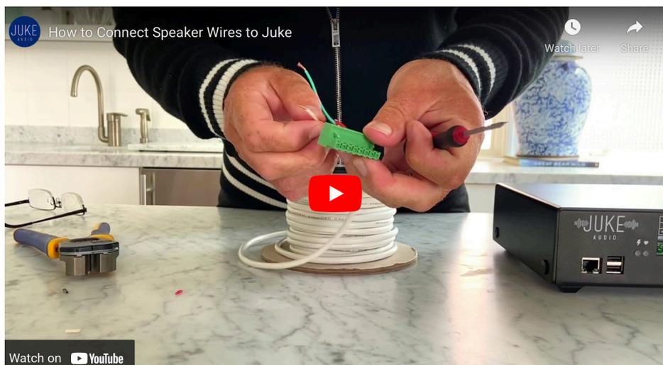
Next connect the speaker wiring. This may require a wire stripper, a small screwdriver, and scissors:
