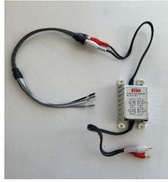
Here is what the wires from the Rockford Fosgate part look like when they are connected in parallel with the left speaker for a zone:
